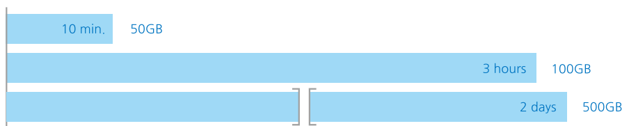
The time that required to encrypt and decrypt large files in gernal ways.
